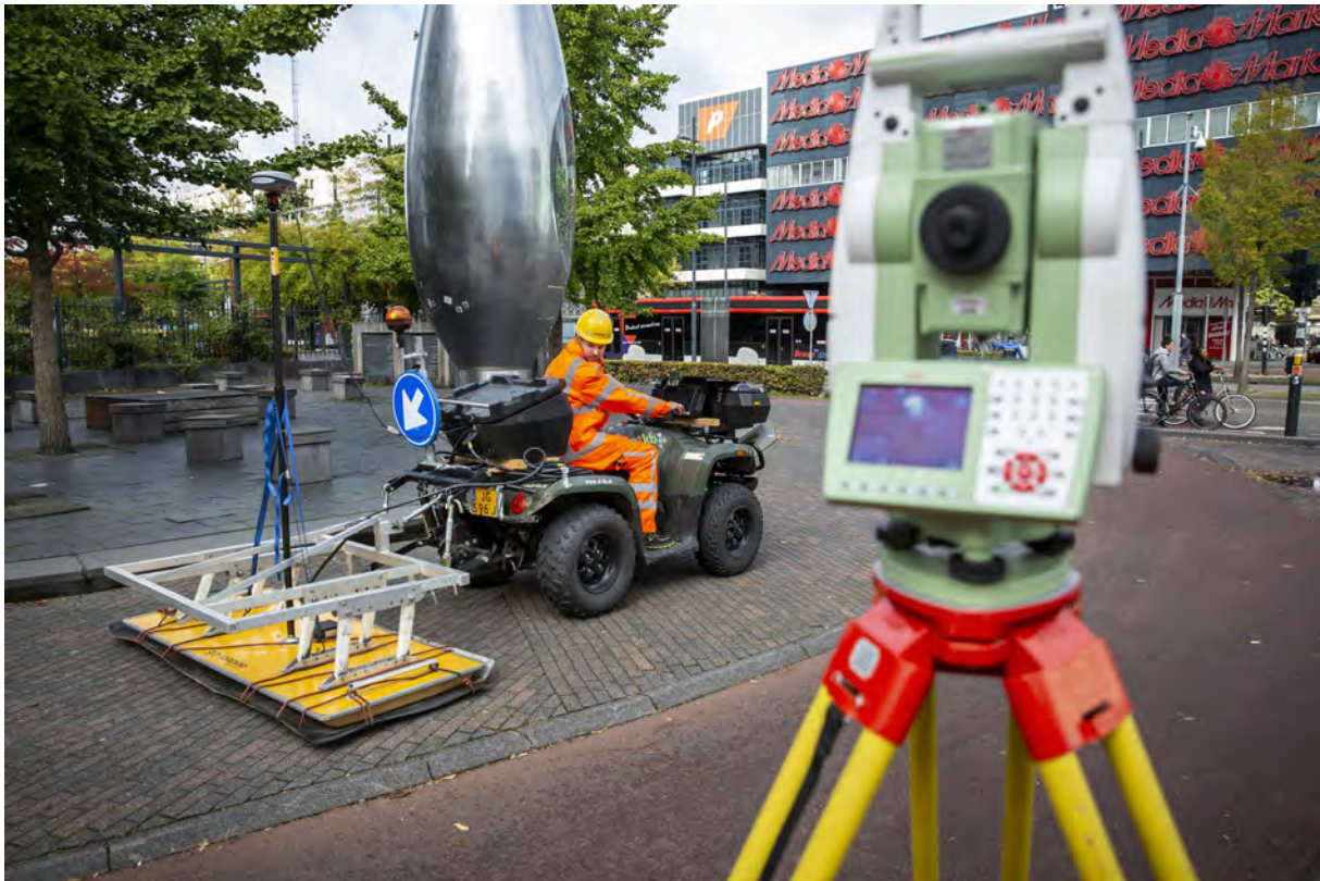
Our geophysics specialists examining the soil using modern measuring equipment and GPS-assisted geophysical surveying technique
